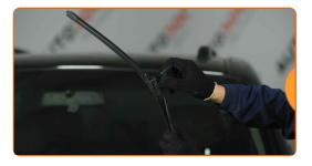
Remove the blade from the wiper arm.
