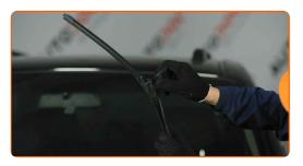
Remove the blade from the wiper arm.
