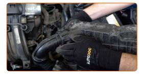
Tighten the clamp fastening the engine air filter housing to the throttle body. Use a flat screwdriver.
