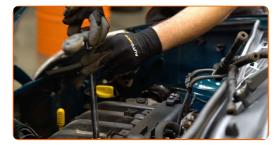
Take out the spark plugs. Use a telescoping magnet.
