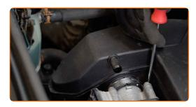
Remove the air filter housing.
