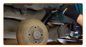
Tighten the top shock absorber fastening. Use a drive socket #16. Use a combination spanner #18. Use a torque wrench. Tighten it to 105 Nm torque.
