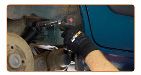
Tighten the lower fastener of the shock absorber. Use a drive socket #16. Use a torque wrench. Tighten it to 105 Nm torque.
