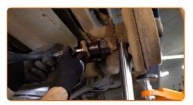
Unscrew the upper fastener of the shock absorber. Use a drive socket #16. Use a combination spanner #18. Use a tap wrench.
