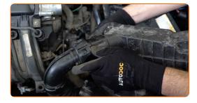
Undo the fastening screws of the air filter cover. Use Torx T25.
