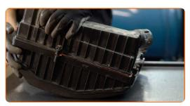
Screw in the fastening screws of the air filter cover. Use Torx T25.
