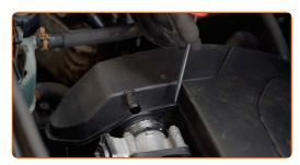
Remove the air filter housing.
