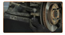
Tighten the tie rod end locknut. Use a combination spanner #19. Use a torque wrench. Tighten it to 44 nm torque.
