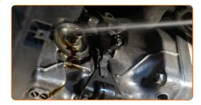
Screw the new filter into its place. Use the 65/14-F socket. Observe the recommended tightening torque.
