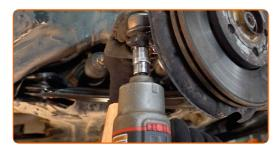
Tighten the fastening nut connecting the tie rod end to the steering knuckle. Use a drive socket #17. Use a torque wrench. Tighten it to 45 nm torque.
