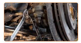
Unscrew the end fastening nut to the steering knuckle. Use a drive socket #17. Use a tap wrench.
