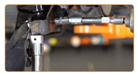
Tighten the lower fastener of the shock absorber. Use a combination spanner #21. Use a drive socket #21. Use a torque wrench. Tighten it to 40 Nm torque.+90°
