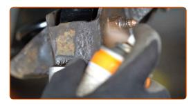
27 Remove the mounting from under the rear axle beam.
