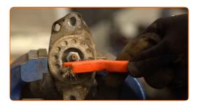
Remove the shock absorber piston rod fastening. Use a combination spanner #16. Use locking pliers.
