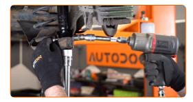
Tighten the top shock absorber fastening. Use a combination spanner #16. Use a drive socket #16. Use a torque wrench. Tighten it to 30 Nm torque.+90°
