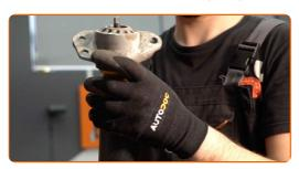
Screw the shock strut piston rod upper fastening. Use a combination spanner #16. Use a drive socket #16. Use a torque wrench. Tighten it to 25 Nm torque.
