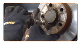
15 Remove the brake disc.
