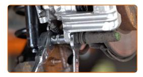
Remove the brake caliper.
