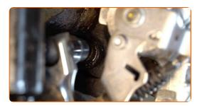
Remove the caliper bracket.
