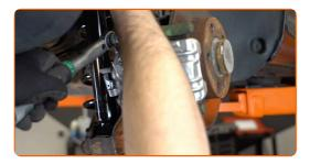
Unscrew the brake hose plug. Use HEX No.H6. Use a ratchet wrench.
