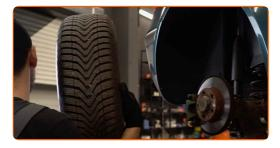
Clean the area where the brake hose is connected to the caliper, and the guide pins area. Use a wire brush. Use a brake cleaner.
