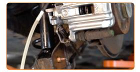
Secure the parking brake cable with the retaining clip.
