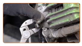
Clamp the brake hose off using a brake hose clamp.
