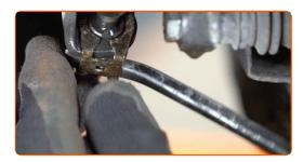
Disconnect the parking brake cable from the caliper. Use water pump pliers. Release the parking brake cable.
