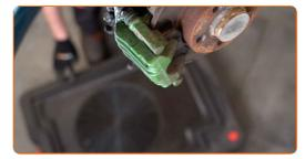
Unscrew the brake hose from the brake caliper. Use a drive socket #13. Use a ratchet wrench.
