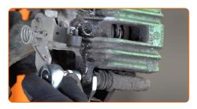
Remove the brake caliper. Use a crowbar.
