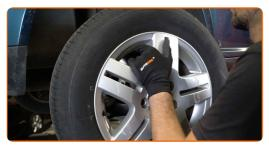
Clean the ABS sensor fastener. Use a nylon cleaning brush. Use WD-40 spray.
