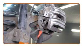
Unscrew the brake caliper bracket fasteners. Use HEX No.H8. Use a ratchet wrench. Use a tap wrench.
