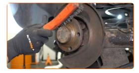
24 Install the brake disc.
