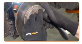
Remove the brake disc.
