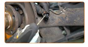
Attach the ABS sensor connector.
