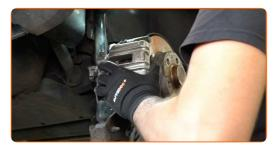
Tighten the brake caliper bracket. Use HEX No.H8. Use a torque wrench. Tighten it to 45 Nm torque.
