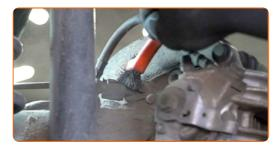
Detach the ABS sensor connector. Use a flat screwdriver.
