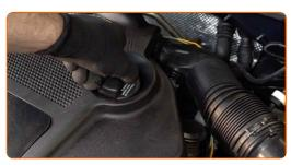
Pour oil into the engine through the filler. Required amount of oil: 4 l.
