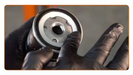
Screw the new filter into its place. Use the 76-14F socket. Use a torque wrench. Tighten it to 18 Nm torque.
