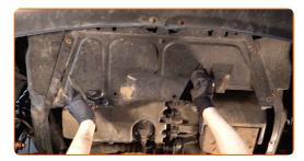
Tighten the fasteners of the oil pan lower cover. Use Torx T20. Use a ratchet wrench.
