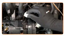
5 Detach the secondary air pump connector.
