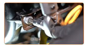
22 Install the secondary air pump.
