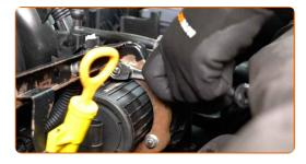
Remove the secondary air pump.
