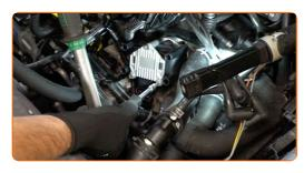
Plug in the ignition coil connector.
