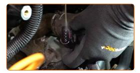
Treat the spark plug wire connectors. Use electronic spray.
