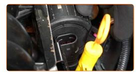
Unscrew the fasteners connecting the secondary air pump to its bracket. Use a combination spanner #10.
