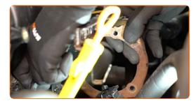
Detach the connector from the ignition coil.
