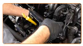
Tighten the fastener of the secondary air pump bracket. Use HEX No.H6. Use a drive socket #13. Use a torque wrench. Tighten it to 9 Nm torque.
