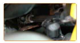
Remove the secondary air pump bracket.
