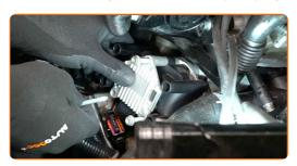
Tighten the ignition coil fastening. Use HEX No.H5. Use a torque wrench. Tighten it to 7 Nm torque.
