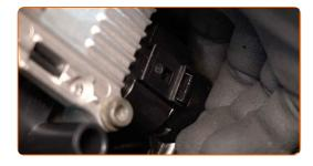
Connect the spark plug wires to the ignition coil.
