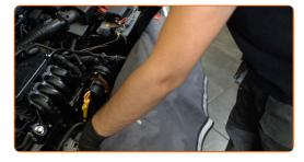
Disconnect the secondary air pump hoses.
