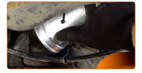
Attach the fuel filter fasteners. Use nippers.
