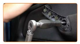
Screw in the lower fasteners of the door card. Use Torx T20. Use a ratchet wrench.
