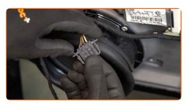
Detach the power window wiring harness. Use a clip removal tool.
