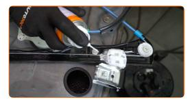
Attach the connector of the central door locking module.
