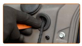
Remove the door panel clips. Use a flat screwdriver.
