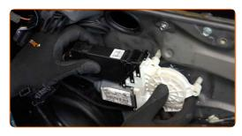
Tighten the fasteners of the power window motor. Use Torx T30. Use a torque wrench. Tighten it to 4 Nm torque.
