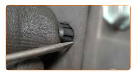
Unscrew the door panel fasteners. Use a drive socket #10. Use a ratchet wrench.
