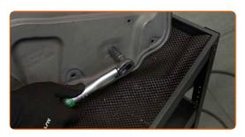
Treat the window regulator drive gear. Use a silicone lubricant.
