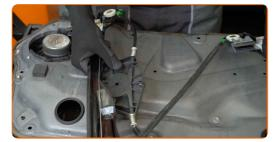
Install the new window regulator mechanism.
