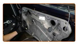
Detach the connector of the central door locking module.
