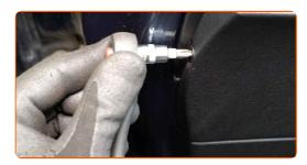
Unscrew the lower fasteners of the door card. Use Torx T20. Use a ratchet wrench.
