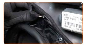
42 Attach the window switch module connectors.
