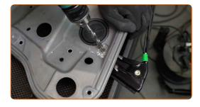
Remove the window regulator mechanism.
