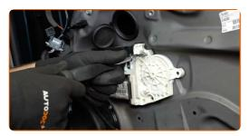
17 Remove the power window motor.
