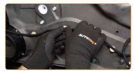
Tighten the door panel fasteners. Use a drive socket #10. Use a torque wrench. Tighten it to 8 Nm torque.
