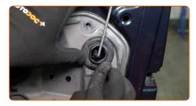
Attach the power window wiring harness.
