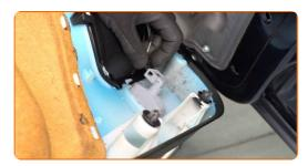
9 Remove the covers from the window raiser fasteners.
