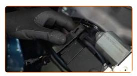
Install the power window motor.
