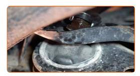
Unscrew the front arm fastener. Use a drive socket #18. Use a ratchet wrench.
