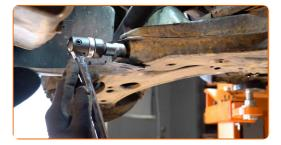
Unscrew the rear arm fastener. Use a combination spanner #18. Use a drive socket #18. Use a tap wrench.
