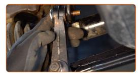
Tighten the fastener connecting the stabilizer link to the stabilizer bar. Use a combination spanner #16. Use a drive socket #16. Use HEX No.H10. Use a ratchet wrench. Use a torque wrench. Tighten it to 15 Nm torque.+90°
