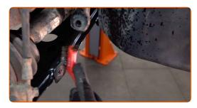
Install a new rod, tighten the fasteners.
