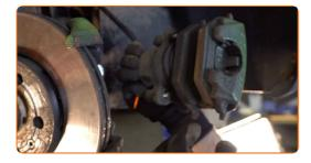
Remove the brake pads. Use a crowbar.
