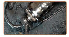
21 Install the brake hose retaining clip. Use a hammer.
