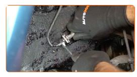
Remove the brake hose retaining clip. Use a crowbar.
