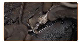
16 Remove the brake hose clamp.
