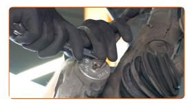
Loosen the fastener connecting the brake pipe to the brake hose. Use a combination spanner #11.
