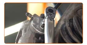
Remove the brake hose clamp.
