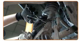
Connect the brake bleeder kit to the brake bleeder screw.
