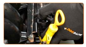
Remove the microfibre cloth from the secondary air pump channels.
