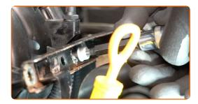
Remove the secondary air pump bracket.
