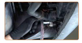
Drain the coolant from the engine.
