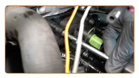
Remove the thermostat housing.
