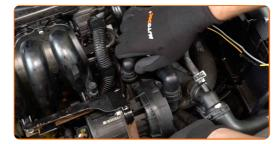
Remove the coolant reservoir cap.
