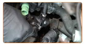
Connect the coolant hoses to the thermostat housing.
