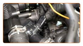
Install the secondary air pump bracket.
