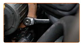
45 Attach the secondary air pump connector.
