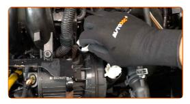
Detach the secondary air pump connector.
