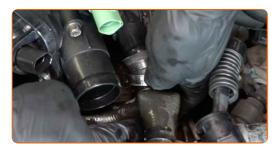
37 Secure the coolant hose clamp. Use a drive socket #7. Use a ratchet wrench.
