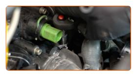
Detach the clamps of the coolant hoses. Use clic-R collar pliers.
