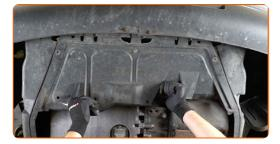
Tighten the fasteners of the oil pan lower cover. Use Torx T25. Use a ratchet wrench.
