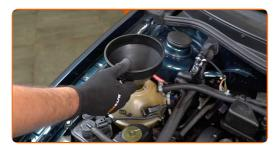
Pour coolant in the coolant reservoir.
