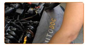
Disconnect the secondary air pump hoses.
