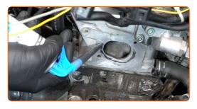
Install the new thermostat housing.
