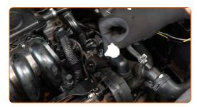
47 Attach the secondary air pump hoses.
