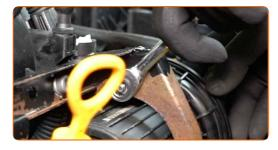
7 Remove the secondary air pump.
