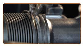
5 Unplug the mass air flow sensor connector.
