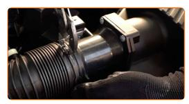
Plug in the mass air flow sensor conntector.
