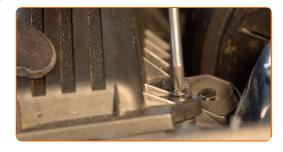
Remove the fender protection cover.
