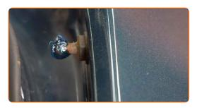
11 Install the new boot lid gas strut.
