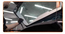
Check the working condition of the boot lid gas springs after they are installed.
