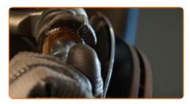
Treat the fastener connecting the tie rod end to the steering knuckle. Use copper grease.
