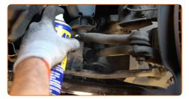
Remove the cotter pin fixing the tie rod end fastening. Use a crowbar. Use round-nose pliers.
