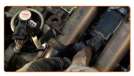
Unscrew the fasteners of the ignition coils. Use a drive socket #10. Use a ratchet wrench.
