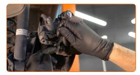
10 Remove the brake caliper.
