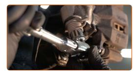
Unscrew the brake caliper fastening. Use a combination spanner #12. Use a combination spanner #17.
