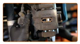
Install the parking brake cable into the brake caliper bracket. Use a rubber mallet. Use a drive socket #17. Use a ratchet wrench.
