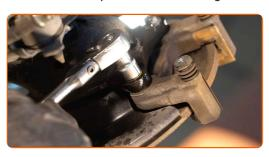
Remove the caliper bracket.
