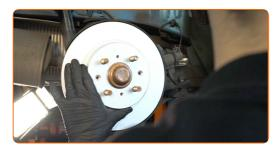
Tighten the brake disc fastening. Use a Phillips screwdriver. Use a torque wrench. Tighten it to 9 Nm torque.
