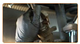
Install the brake caliper and fix it. Use a combination spanner #12. Use a combination spanner #17. Use a drive socket #12. Use a torque wrench. Tighten it to 23 Nm torque.
