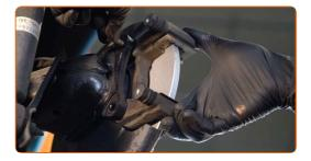
Tighten the brake caliper bracket. Use a drive socket #14. Use a torque wrench. Tighten it to 55 Nm torque.
