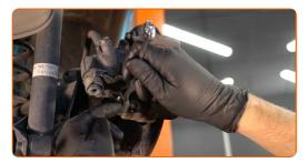
10 Remove the brake caliper.
