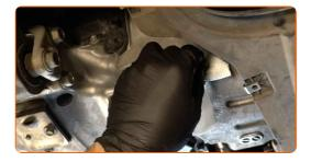
Screw in the new drainage plug and tighten it. Use a drive socket #17. Use a torque wrench. Tighten it to 27 Nm torque.
