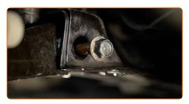
Install the rear fastener of the control arm. Use a drive socket #19.
