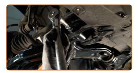
Tighten the rear fastener of the control arm. Use a drive socket #19. Use a torque wrench. Tighten it to 93 nm torque.
