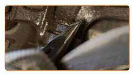
Unscrew the ball joint fastening to the steering knuckle. Use a combination spanner #19.
