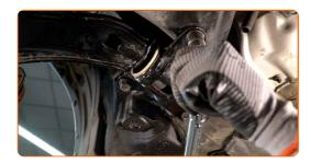
Tighten the fasteners of the ball joint. Use a combination spanner #22. Use a torque wrench. Tighten it to 65 nm torque.
