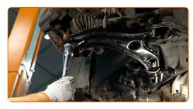
Screw the rear fastener connecting the control arm to the subframe. Use a drive socket #19.
