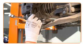
Disconnect the lower arm from the steering knuckle. Use a ball joint puller.
