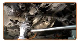
Remove the rear fastener of the control arm. Use a drive socket #19.
