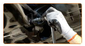
Unscrew the rear fastener connecting the control arm to the subframe. Use a drive socket #19. Use a tap wrench.
