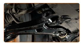
Screw the front arm fastener. Use a drive socket #19.
