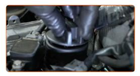
Tighten the oil filler cap.
