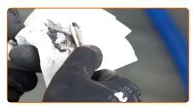
Lubricate guide pins with special brake grease.
