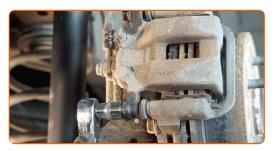
10 Remove the brake caliper.
