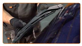
Remove the blade from the wiper arm.
