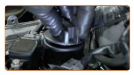
Tighten the oil filler cap.
