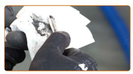
Lubricate guide pins with special brake grease.
