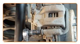
10 Remove the brake caliper.
