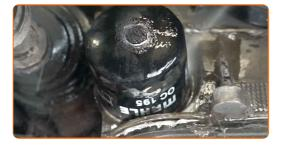
Unscrew the oil filter. Use the 65-14F socket. Use a ratchet wrench.
