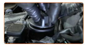
Tighten the oil filler cap.
