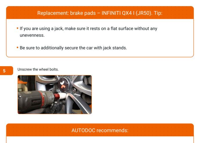
• Warning! To avoid injury, hold the wheel while unscrewing the fastening bolts. INFINITI QX4 I (JR50)
