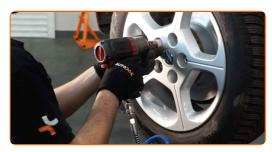
Lower the car and working in a cross order, tighten the wheel bolts. Use a torque wrench. Tighten it to 108 Nm torque.
