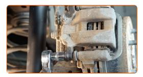
10 Remove the brake caliper.
