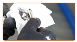
Lubricate guide pins with special brake grease.
