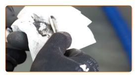
Lubricate guide pins with special brake grease.
