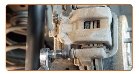
10 Remove the brake caliper.
