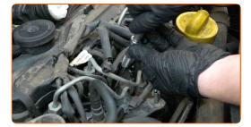
Tighten the glow plugs. Use the spark plug socket #10. Use a torque wrench. Tighten it to 15 nm torque.
