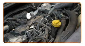
Detach the glow plug wiring connectors.
