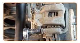
10 Remove the brake caliper.
