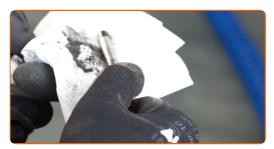
Lubricate guide pins with special brake grease.
