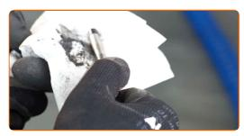
Lubricate guide pins with special brake grease.
