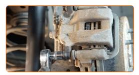
10 Remove the brake caliper.
