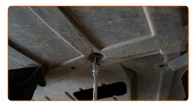
Remove the oil pan cover. Use a drive socket #10. Use a flat screwdriver.
