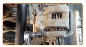
10 Remove the brake caliper.
