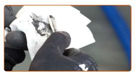
Lubricate guide pins with special brake grease.
