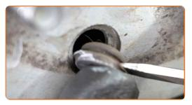
Release the parking brake adjuster. Use a flat screwdriver.
