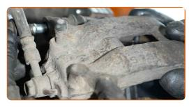
Install the brake caliper guide pins.
