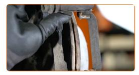
Remove the rubber plug. Use a flat screwdriver.
