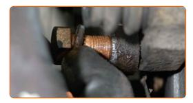
Tighten the brake caliper bracket fasteners. Use a drive socket #19. Use a torque wrench. Tighten it to 80 nm torque.
