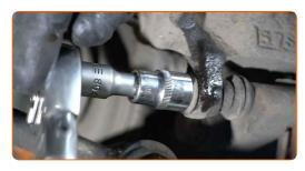
Remove the brake caliper guide pins.
