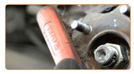
Treat the contacting surface. Use ceramic grease.
