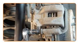
10 Remove the brake caliper.
