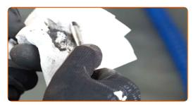
Lubricate guide pins with special brake grease.
