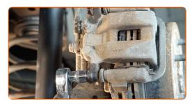
10 Remove the brake caliper.
