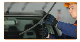
Remove the blade from the wiper arm.
