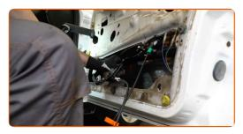
Tighten the fasteners of the window regulator assembly. Use a drive socket #10. Use a torque wrench. Tighten it to 10 Nm torque.
