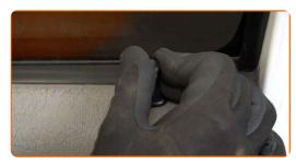
Screw in the door handle fastener. Use a Phillips screwdriver.
