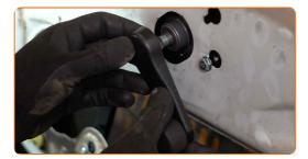
Set the window regulator assembly into the fully lowered position.
