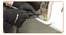
Remove the window regulator mechanism.
