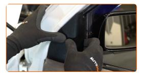
Attach the wing mirror adjustment handle.
